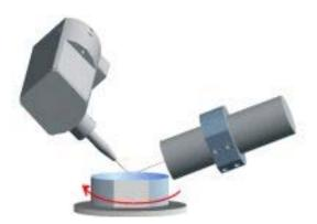
The Omega-scan principle. The X-ray source and detector have fixed angles and is not moving. The sample to be measured is rotated ( $\Omega$ ) and because of the geometry multiple diffraction peaks are being recorded in one revolution. One revolution takes 5 seconds, after which the compete crystal structure can be computed.
