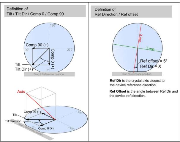
Output from the combined XRD and geometrics measurement. The Stop/Reference position can be a notch or flat
