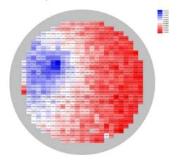
Results from a combined  $\Omega$ -scan/ $\Theta$ -2 $\Theta$  crystalline analysis across a polished 150mm Si (001) Wafer
